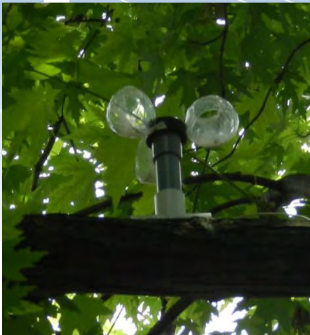
Anemometer provides linear voltage signal (above)
