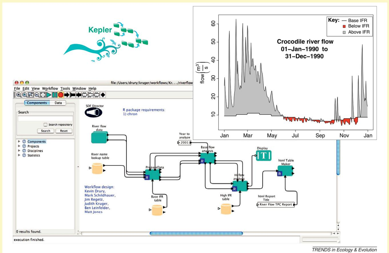
**Figure 1.** The Kepler scientific workflow system can be used to capture a complete analytical procedure, even when multiple statistical analysis and modeling systems are in use. This scientific workflow encapsulates all of the processes used to model and visualize water flow characteristics over time, and effectively communicates periods when system thresholds have been exceeded so that adaptive management processes can be employed.
